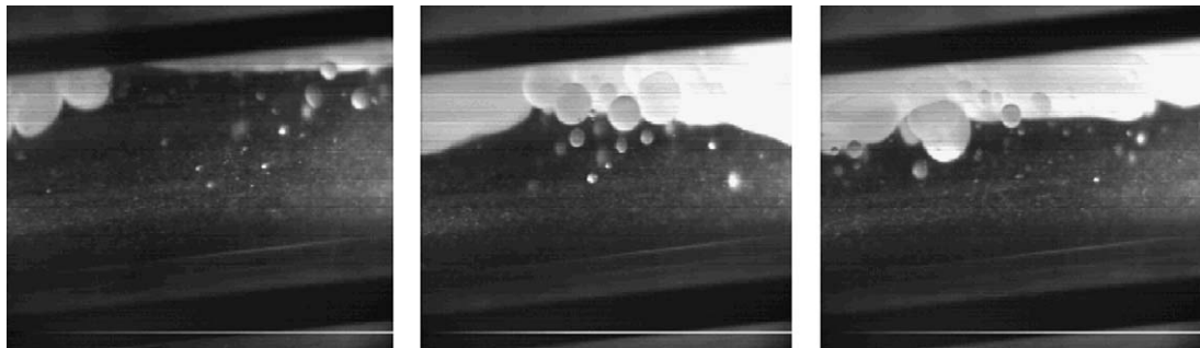
Fig. 5. Plug flow (PG) at +5° inclination, 0.7 m/s mixture velocity and 10% input oil fraction.
